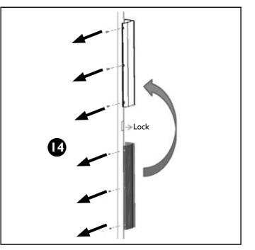
**14** As the door has turned 180 degrees, reposition your handle above the lock (Full Glass and Black Piano doors only): Unscrew the six screws placed on the side of the door, using the Allen wrench (2,5 mm), which you will find in the handle's box.
