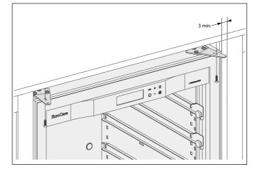
• Use the correct screws to secure the wine cabinet under the work surface or in the unit through the holes provided in the hinges.
